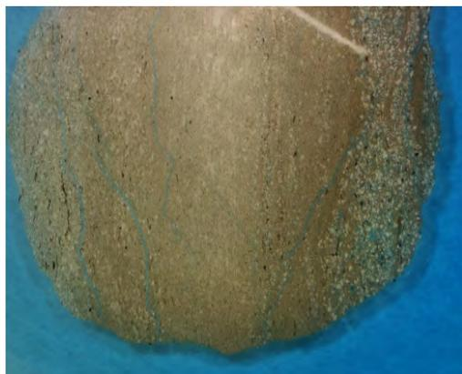
Fig. 5. A failed shale sample from Fig 4.
