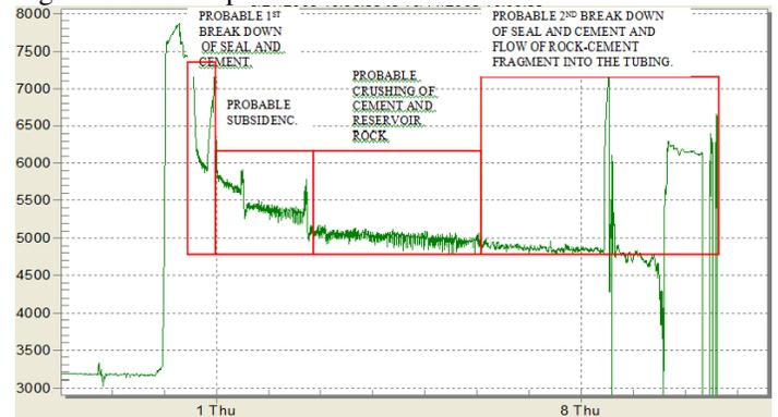
Fig. 14. The “C” sand production record.
