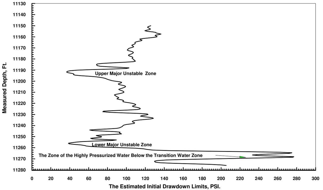
Figure 14. Measured Depth VS The Model-Derived Estimates of Initial Drawdown in Well (1).
