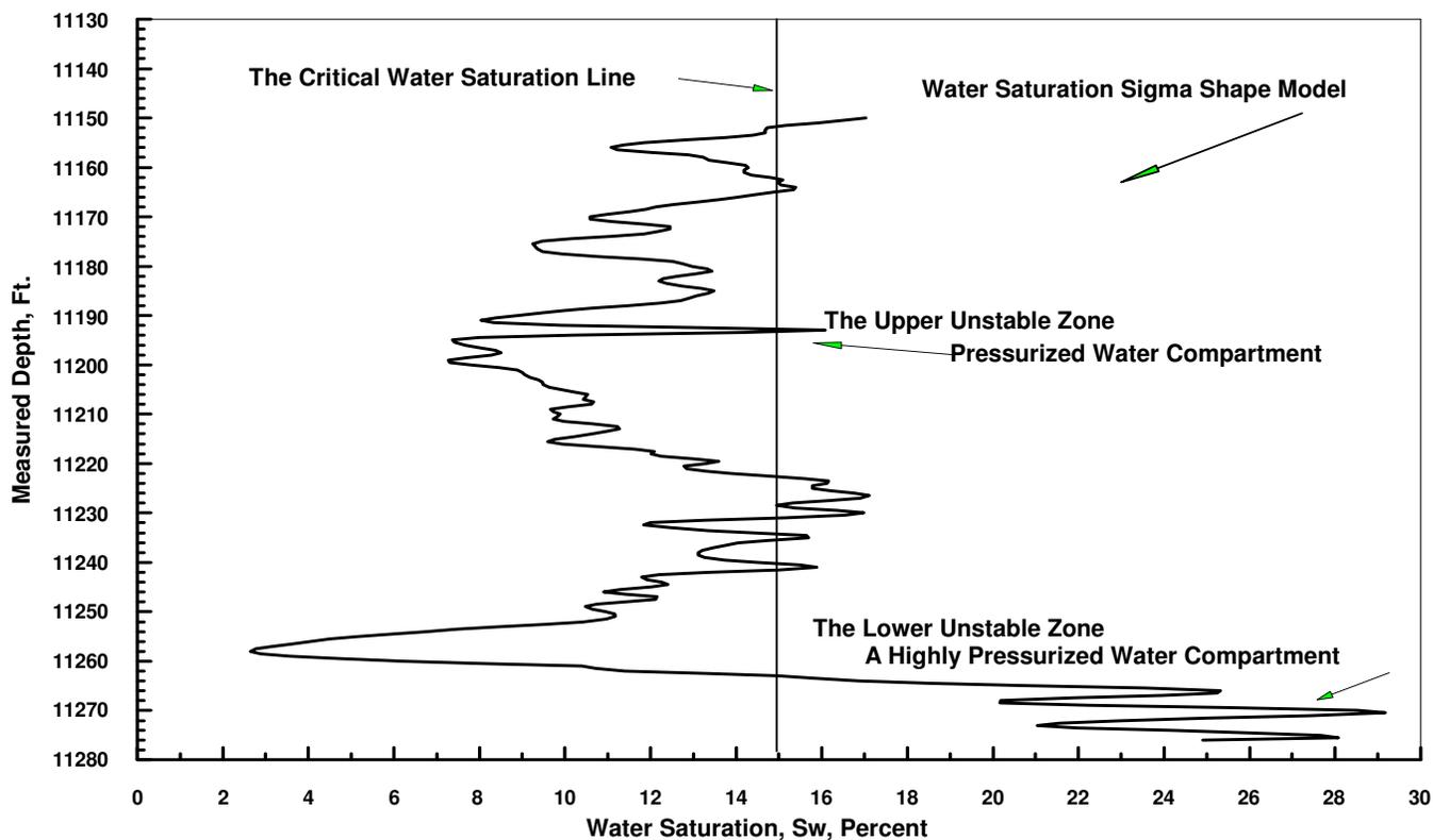
Figure 16. Measured Depth VS Model-Derived Water Saturation in Well
