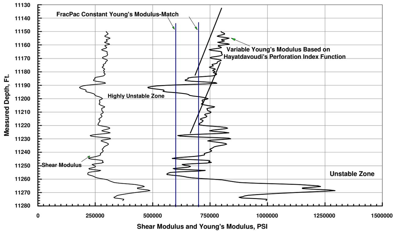
Figure 12. Measured Depth VS Log Derived Estimates of Rock Mechanical Properties in Well (1).
