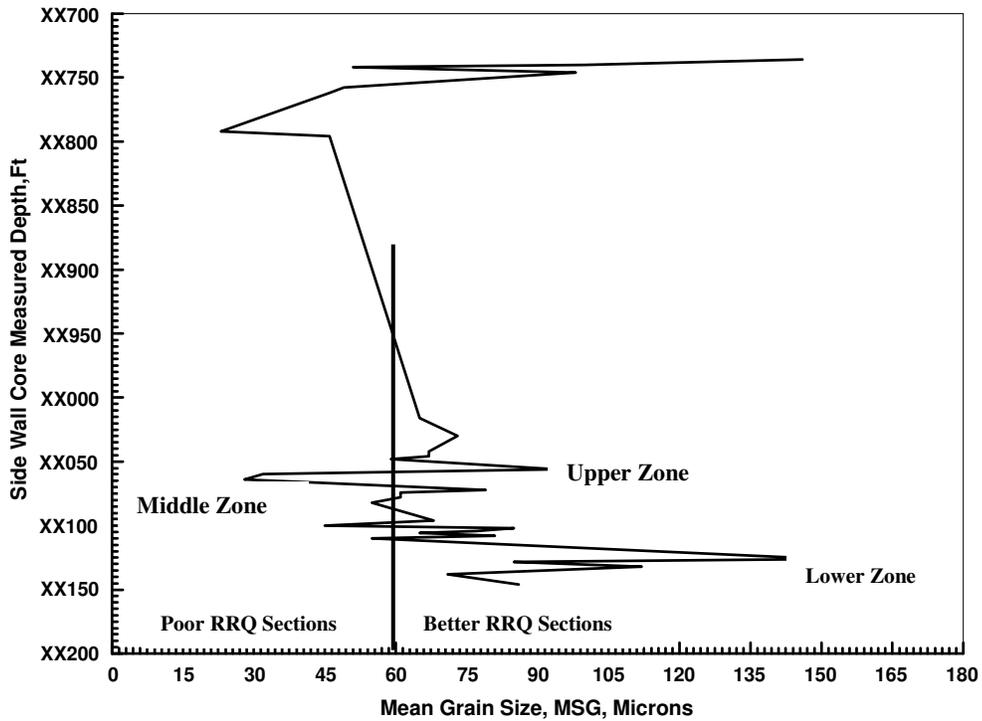
Figure 7. An Example of Measured Depth, MD, VS Mean Grain Size, MGS. Note the Grain Coarsening Downward Trend in Well (2).
