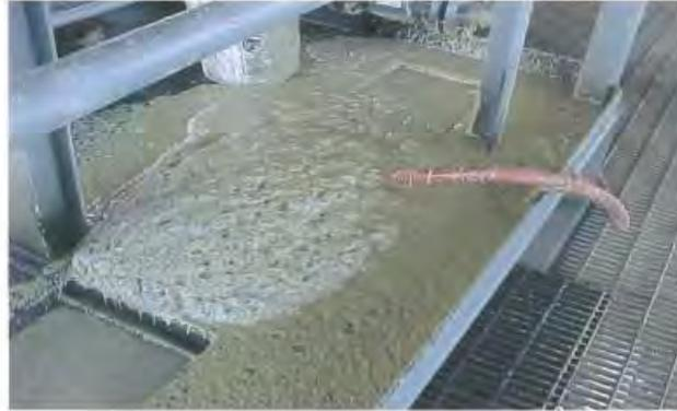
Figure 4. Liquefied Sand Flows Can Bring Production to a Halt.
