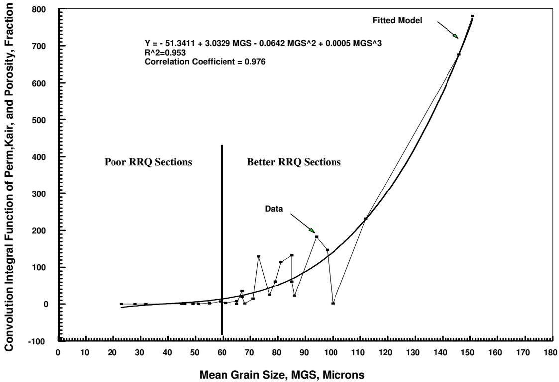
Figure 6. Convolution Integral Function Values of Side Wall Core Permeability,  $K_{air}$ , and Porosity,  $\phi$ , (fraction) VS Mean Grain Size, MGS, An Example of Turbidite Sand Characterization in Well (2). Note the effect of the Downward Coarsening trend of the MGS on  $K$ ,  $\phi$ , and possibly, the Reservoir Rock Quality, RRQ, and the Completion Interval stability
