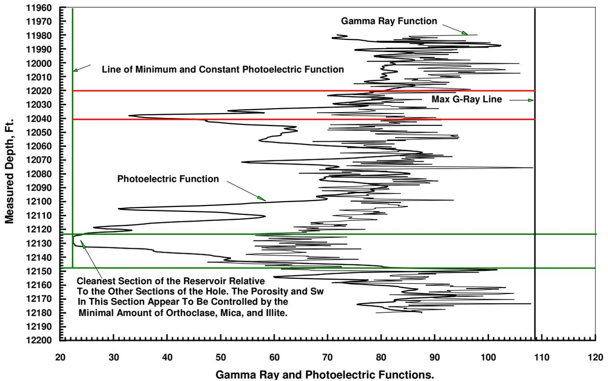
Figure 27. Measured Depth VS Gamma Ray and Photoelectric Functions in Well (2).
