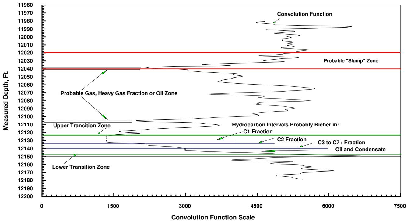
Figure 25. Measured Depth VS Convolution Function in Well (2).
