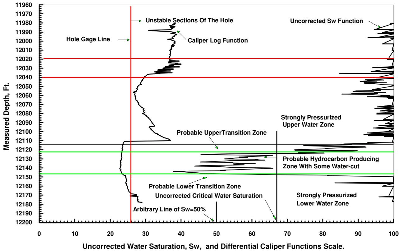
Figure 32. Measured Depth VS Uncorrected Water Saturation a Differential Caliper Functions in Well (2).
