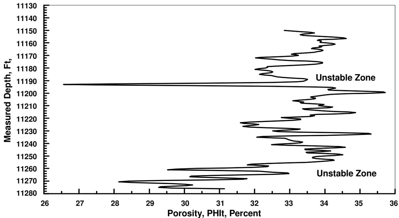
Figure 15. Measured Depth VS Log-Derived Estimates of Uncorrected Porosity in Well (1).
