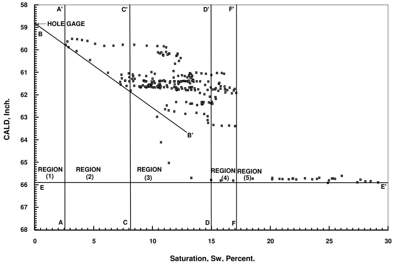
Figure 19. Caliper Log Function Values VS Water Saturation in Well (1). Note how the 'S' shape function defines the *unstable borehole* regions 4 and 5, transition zone 3, and the *stable* region 2.
