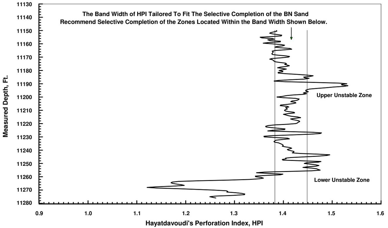
Figure 13. Measured Depth VS HPI Model for Selective Completion in Well (1).
