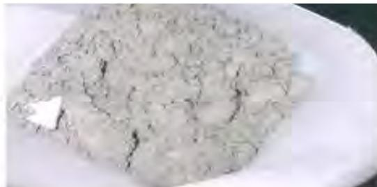
Figure 5. A Sample of Dried, Liquefied Sand. This sample may flow again upon addition of some small amount of water
