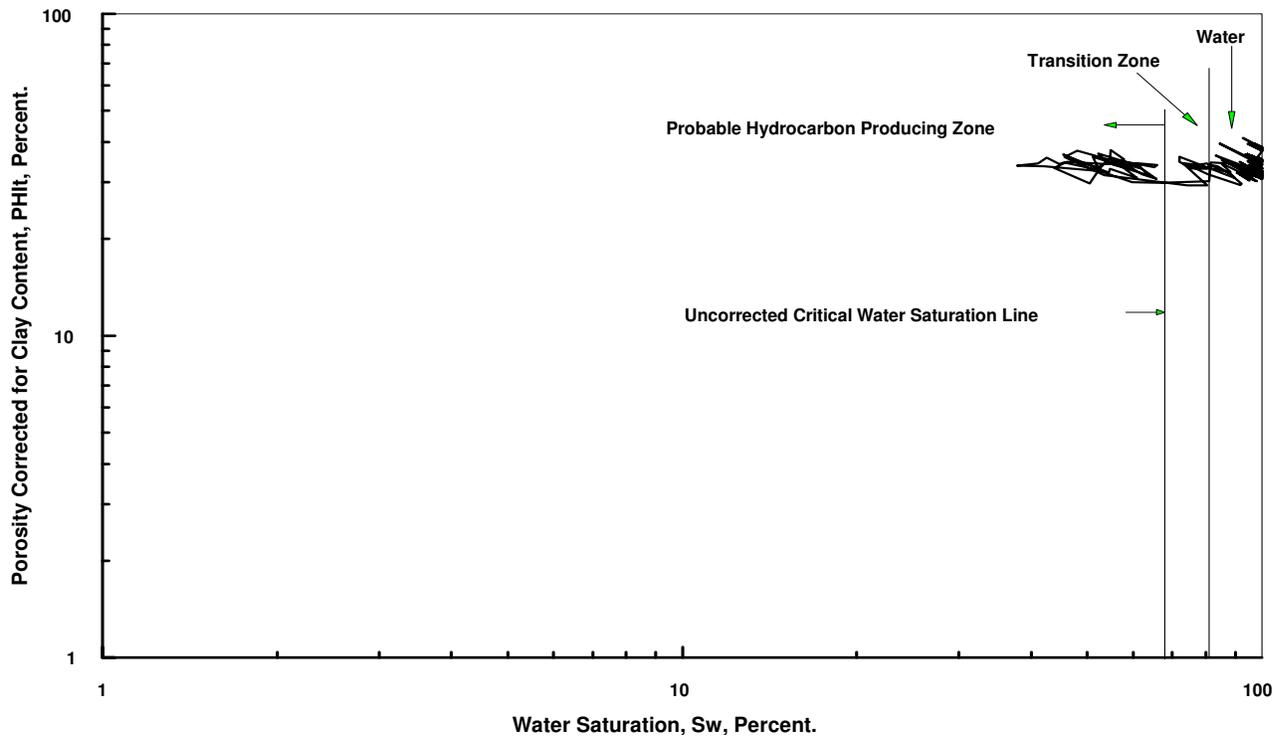
Figure 20. Corrected Porosity VS Water Saturation in Well (2). Compare this figure with Figure 17 and note the difference in Water Saturation of two wells.
