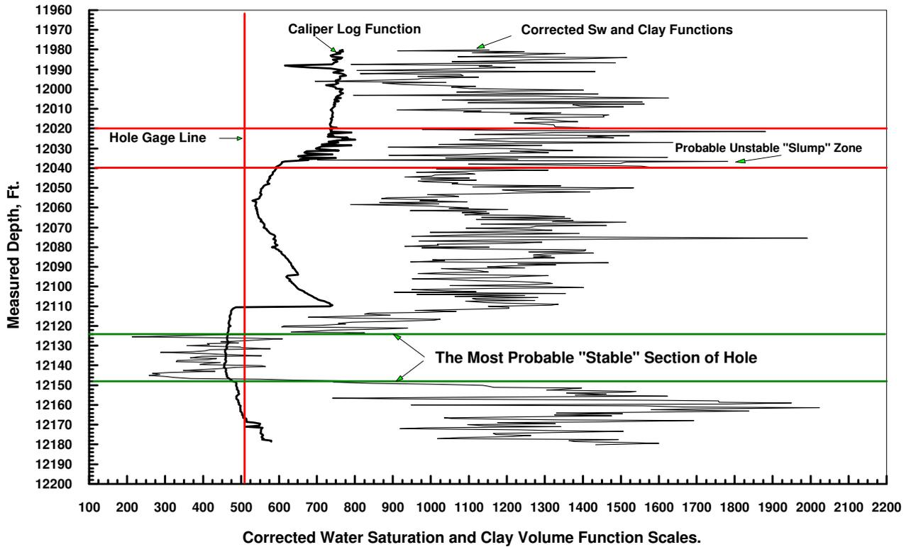
Figure 35. Measured Depth VS Corrected Water Saturation and Clay Volume Functions in Well (2).
