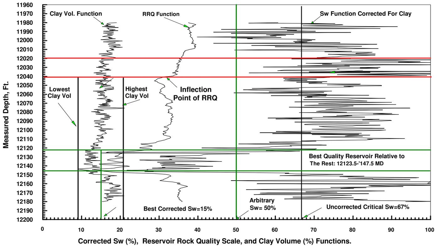
Figure 28. Measured Depth VS Reservoir Rock Quality (RRQ) and Clay Volume Functions in Well (2).
