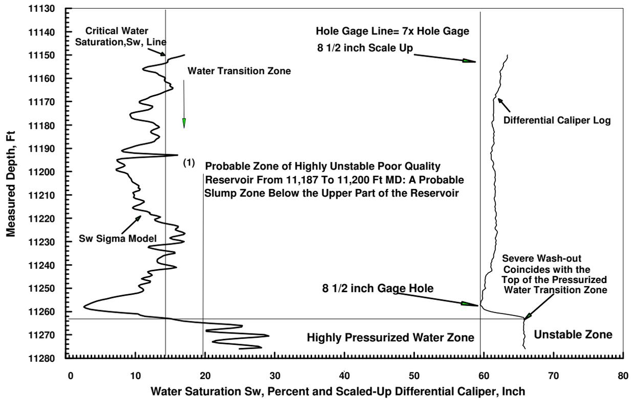
Figure 18. Measured Depth VS Water Saturation and Differential Caliper Log in Well (1).
