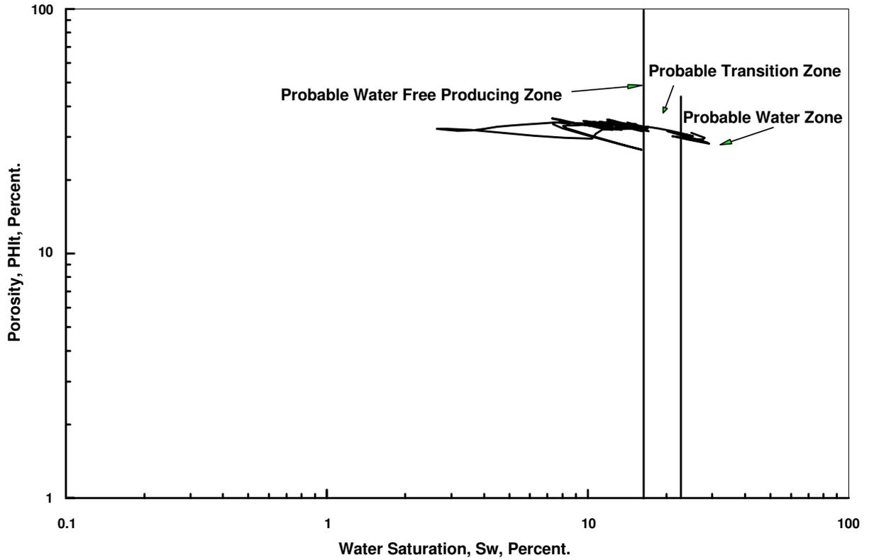
Figure 17. Log-Derived Porosity VS Water Saturation in Well (1).
