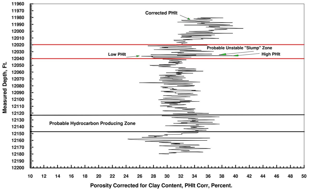
Figure 30. Measured Depth VS Corrected Porosity for Clay Content in Well (2).
