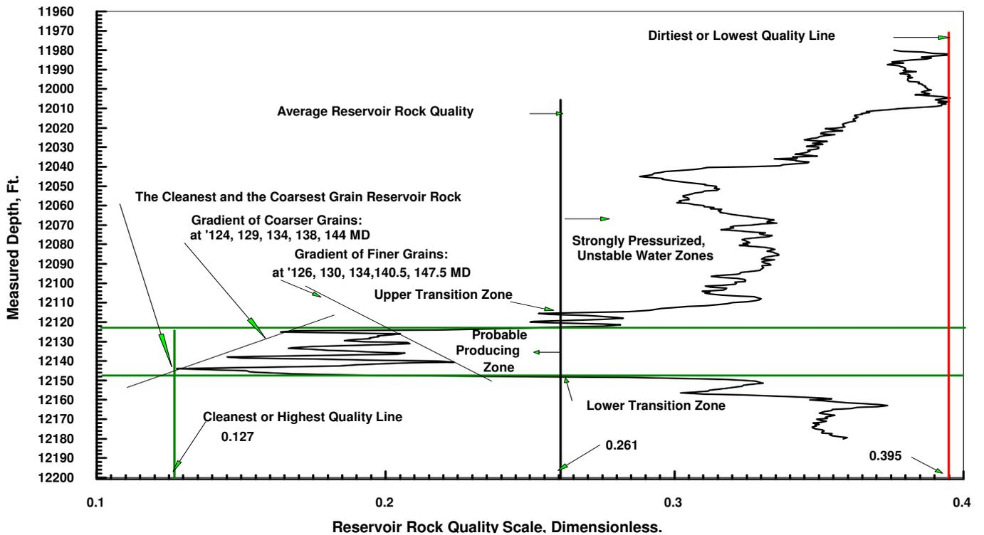
Figure 29. Measured Depth VS Reservoir Rock Quality in Well (2). Compare this figure with Figures (6) and (7) and note how the gradient of coarser sand grains control the Reservoir Rock Quality, (RRQ).
