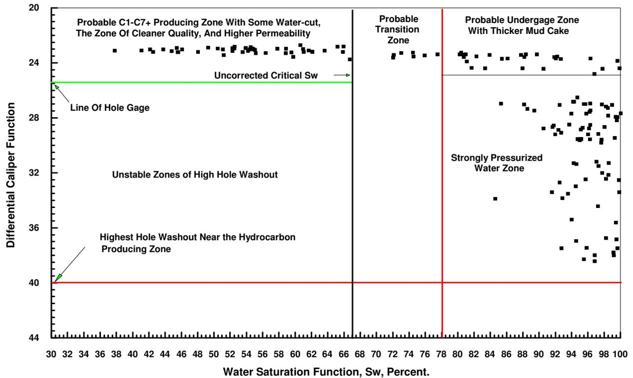
Figure 31. Differential Caliper Function VS Water Saturation Function in Well (2). Note how these functions generate a plot similar to the plot of Capillary Pressure VS Water Saturation.
