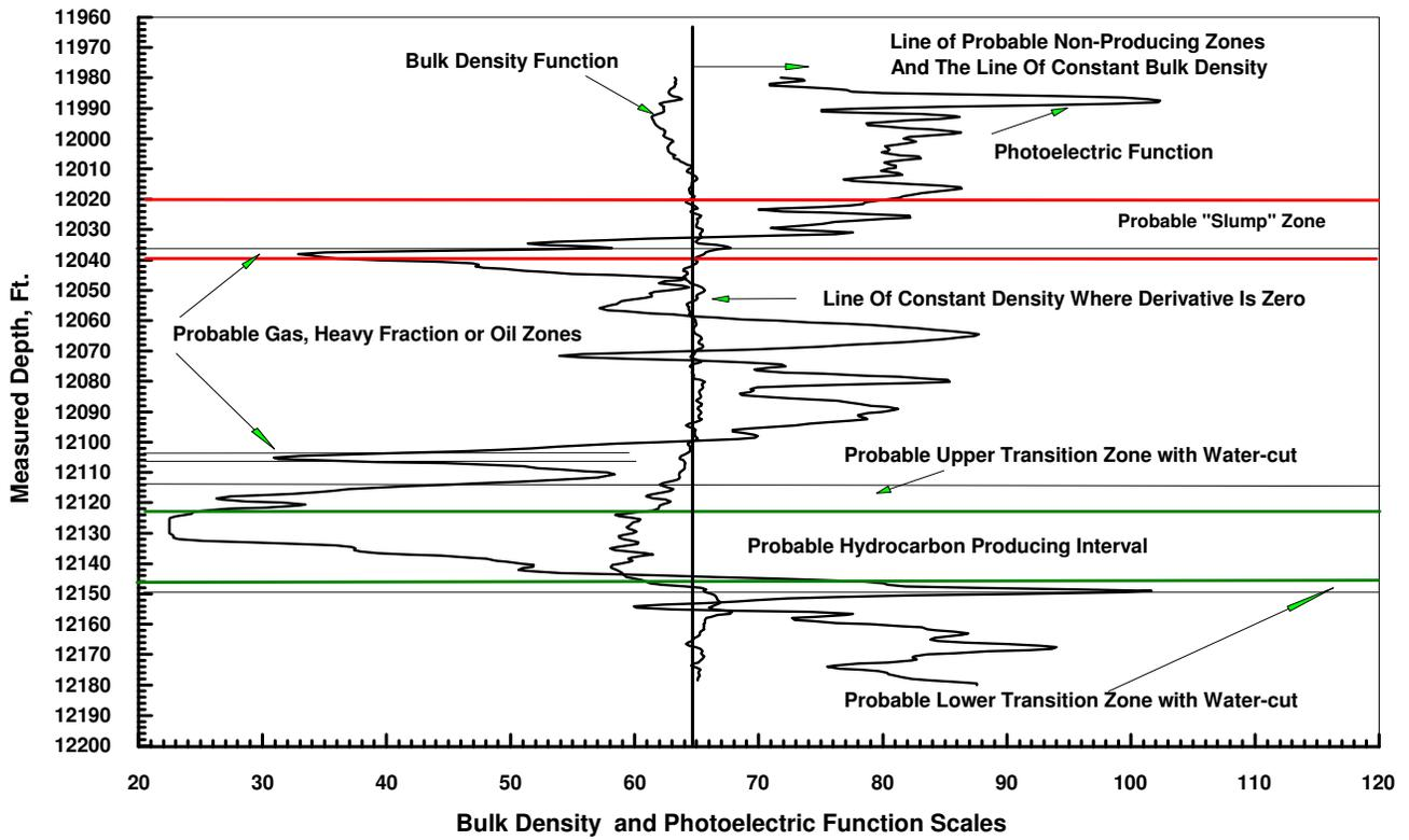
Figure 24. Measured Depth VS Bulk Density and Photoelectric Functions in Well (2).
