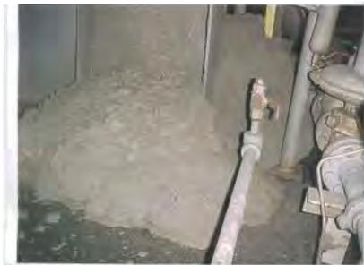
Figure 1. Liquefied Sand Produced From Well (1).
