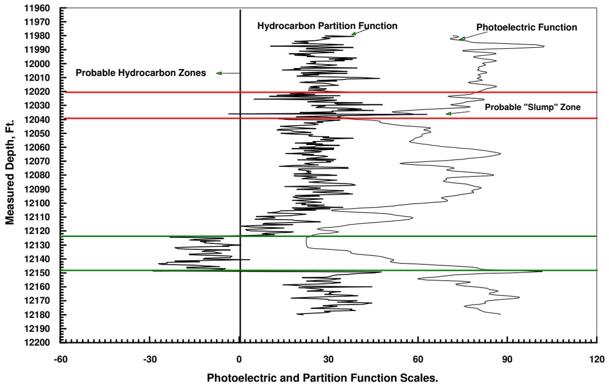
Figure 23. Measured Depth VS Photoelectric and Partition Functions in Well (2).
