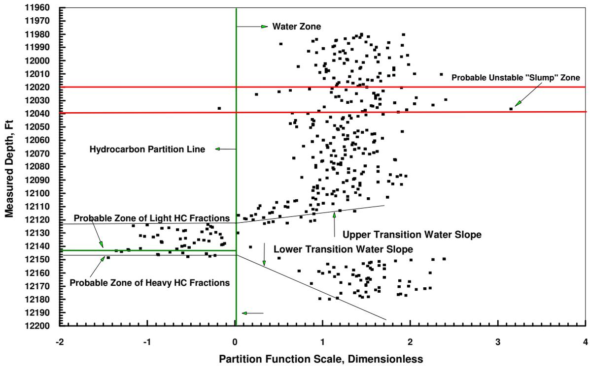
Figure 22. Measured Depth VS Partition Function. Note the existence of two separate water zones with two distinct upper and lower slopes in Well (2).
