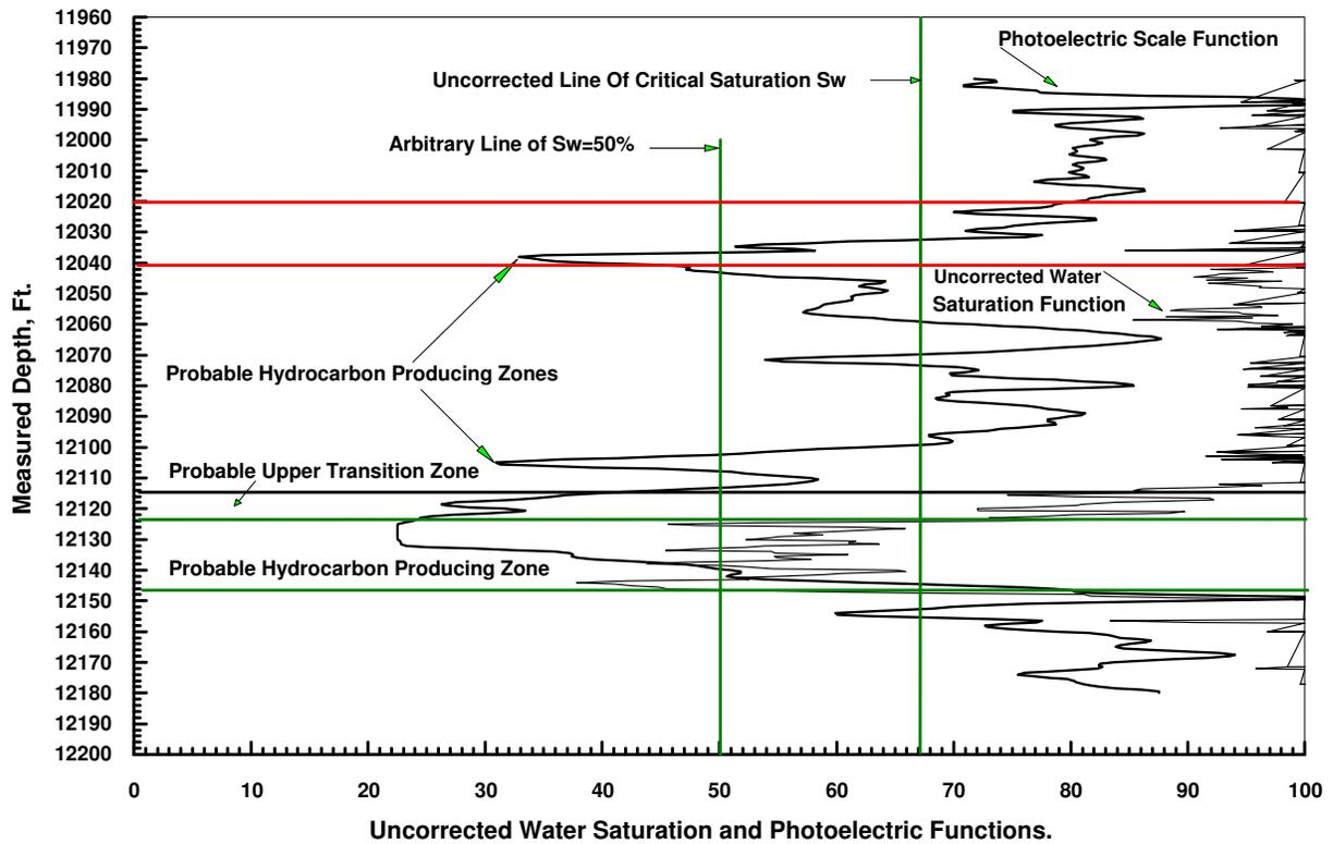
Figure 26. Measured Depth VS Uncorrected Water Saturation and Photoelectric Functions in Well (2).
