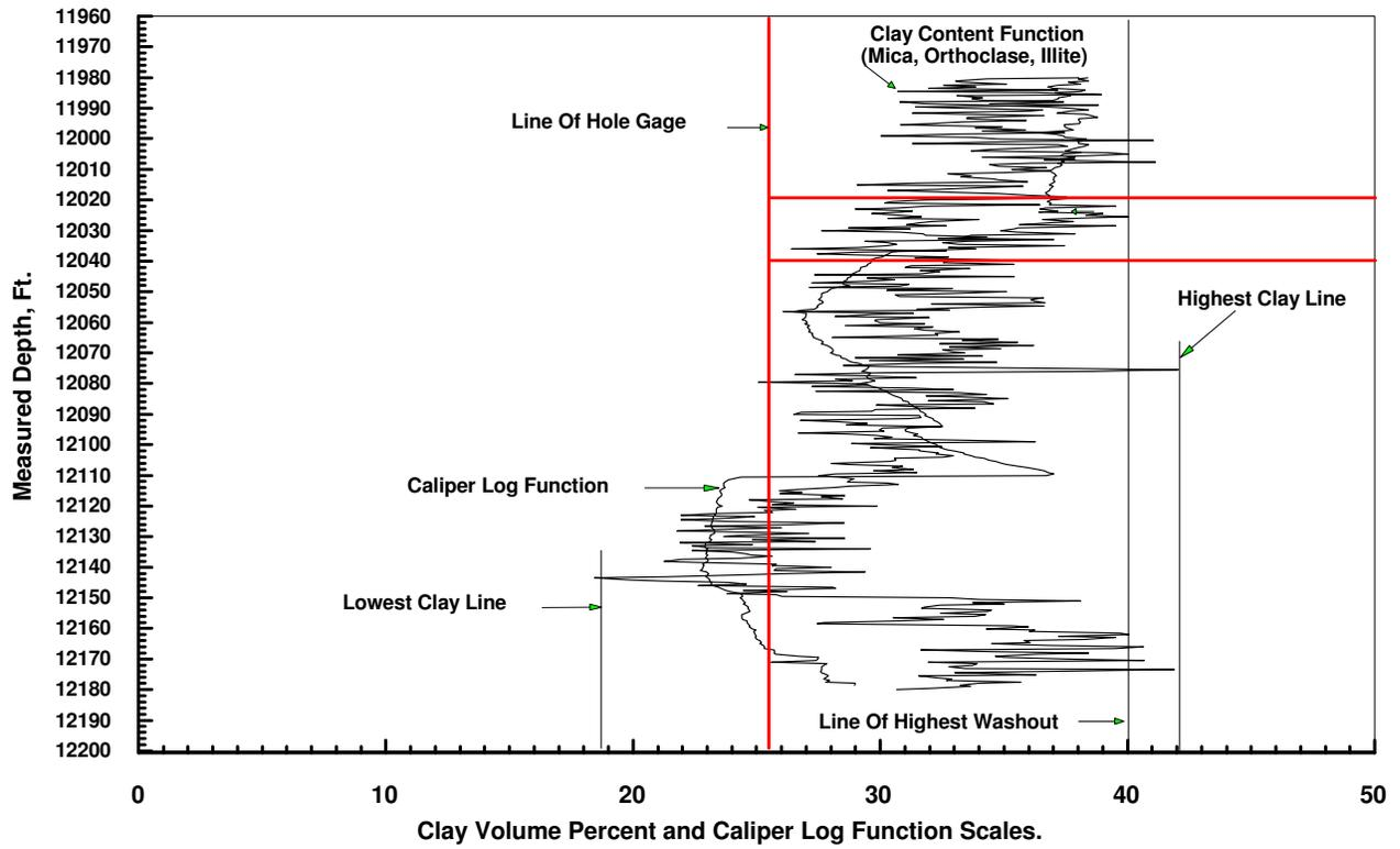
Figure 34. Measured Depth VS Clay Volume and Caliper Log Functions in Well (2).
