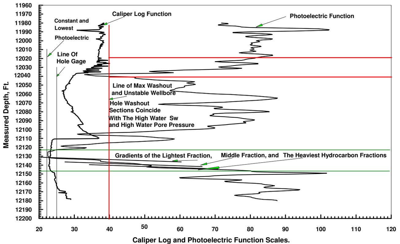
Figure 33. Measured Depth VS Caliper Log and Photoelectric Functions in Well (2).
